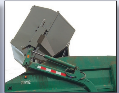
Auto release unloading door.
