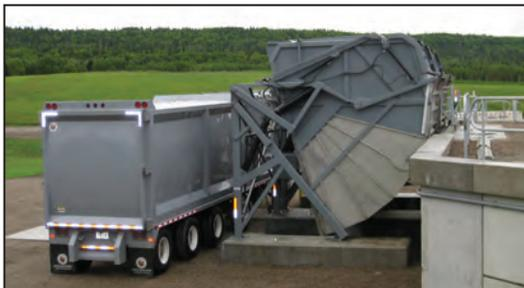
Integrates with walking floors and compaction trailers.
